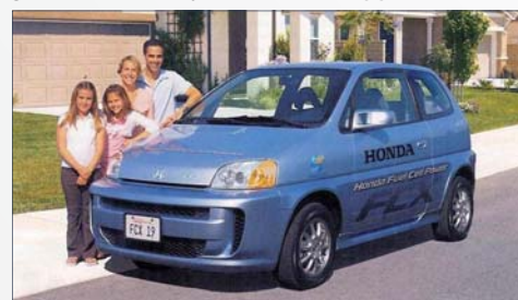
Figure 3: Honda recently began leasing its Fuel Cell car in California. It has a 270-mile range with an efficiency equivalent to 74 miles per gallon. Water is the only emission from its tailpipe.
